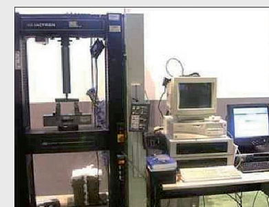
Testing of interlaminar and intralaminar shear strength
