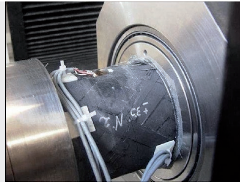
Testing of interlaminar and intralaminar shear strength
